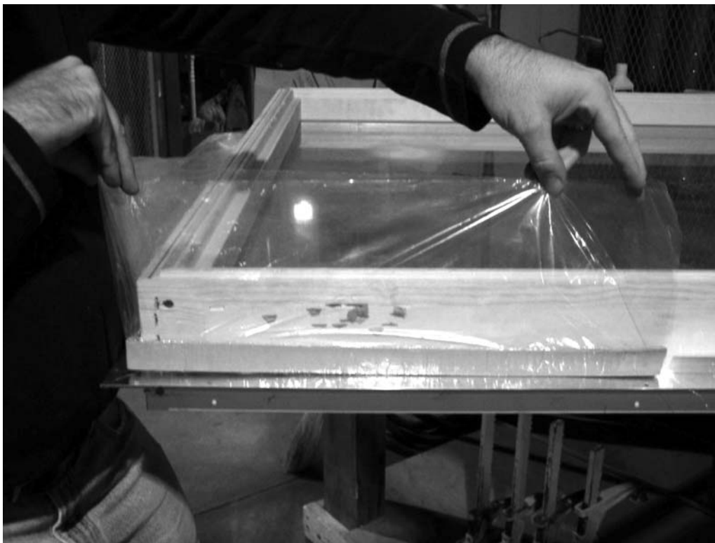
FIG. A1.7 Type B Material Applied to Window Frame
