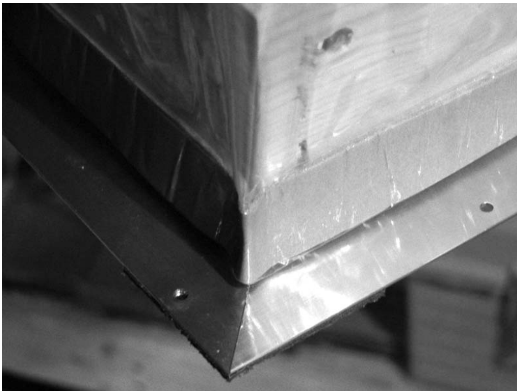
FIG. A1.7 Type B Material Applied to Window Frame
