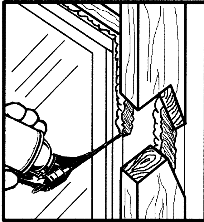
FIG. A1.4 Optional Second Bead Approach for Type A Material
