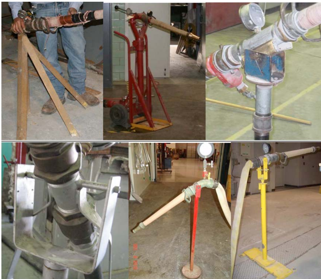
FIG. 2 Typical Hose Mounting Methods
