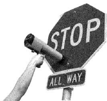
FIG. 3 Portable Retroreflectometer Positioned for Photometry of Sign Face
