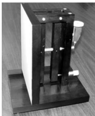
FIG. 9 A shearography camera calibration device consists of a means to apply a known deformation to an aluminum flat plate. The flat surface deformation is imaged. This device allows verification of the shearography camera operation, laser stability, and the minimum coherence length.
