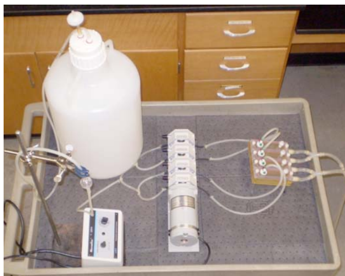
FIG. 2 Drip Flow Reactor Laboratory Set-Up in Continuous Flow Operation
