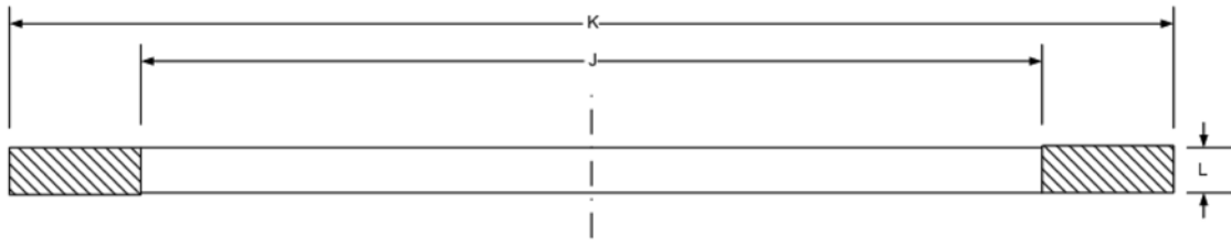
FIG. 3 Knife-Edge Gasket Dimensions
