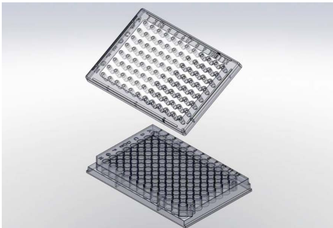
96-well tissue culture plate (bottom) and corresponding 96-peg lid (top).
