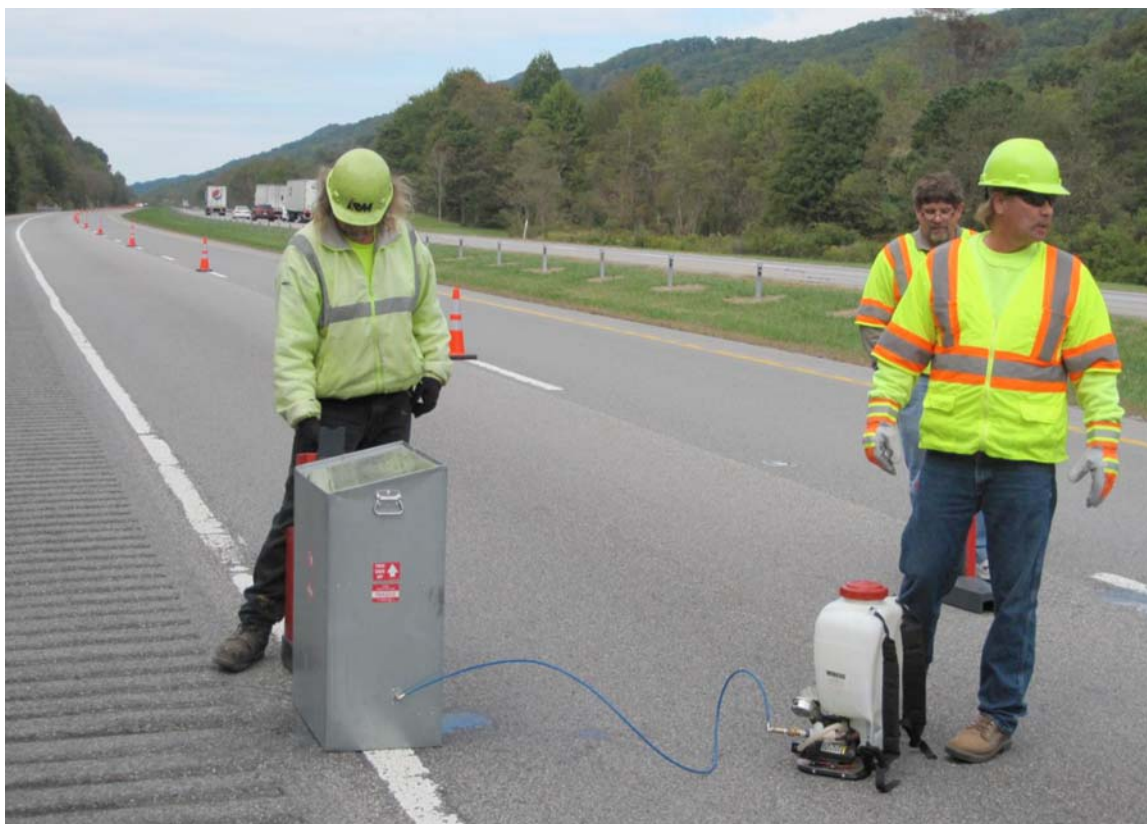
FIG. A1.9 Fabricated Wetting Device in Use
