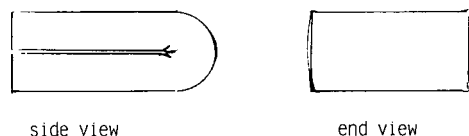
Flattened bend - collapsed eye of the bend
