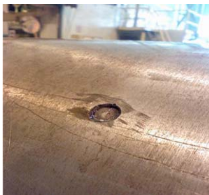
FIG. X2.2 (Reference Fig. X2.1. One circumferential crack on the ID was ~6 mm [ \frac{1}{4} in.] long. The other crack on the OD was ~12 mm [ \frac{1}{2} in.] long.
