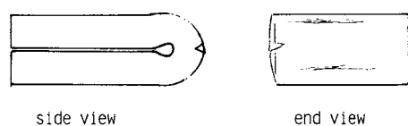
Flattened bend - outer surface and edge cracks
