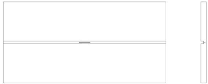
FIG. 4 Flat Plate Sample Serial Number XXX Showing Size and Location of Reference Notch (Plan View and Side View. Not to Scale)
