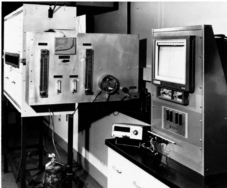
FIG. X2.1 Historic Photograph of Flooring Radiant Panel Tester Apparatus
