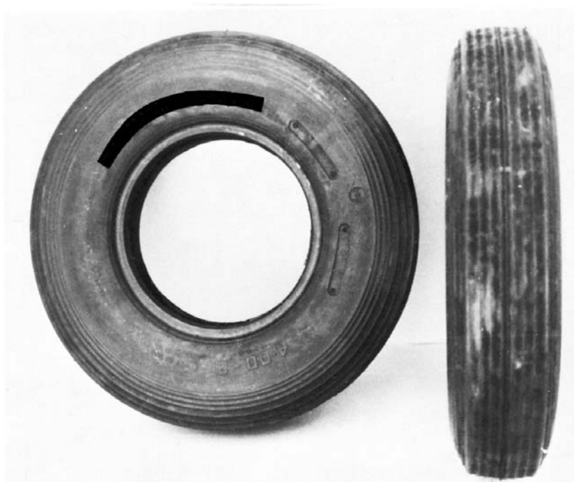
FIG. A1.1 Mu-Meter Test Tire
