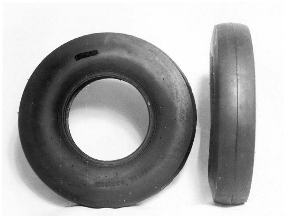
FIG. A2.1 Alternate Mu-Meter Tire
