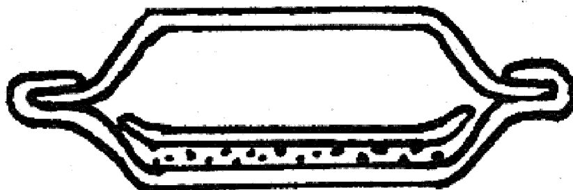
FIG. 2 Sample Pan Collapsed and Collected
