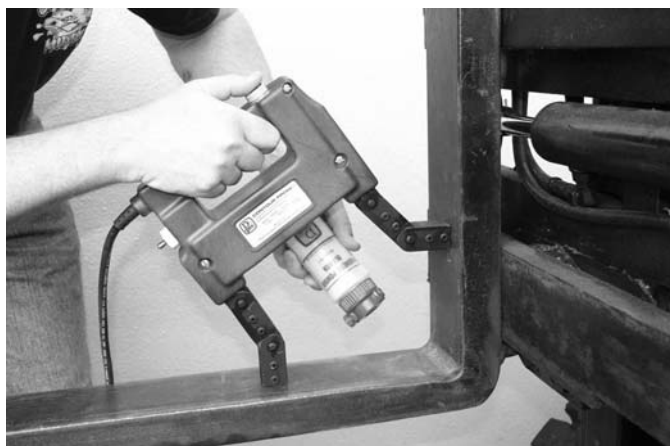
FIG. 1 Yoke Method of Part Magnetization
