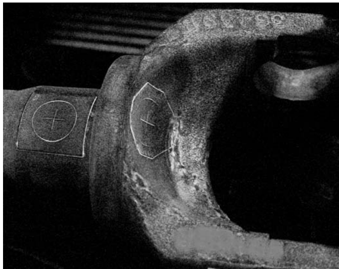
FIG. A1.6 Yoke Showing Balanced QQIs
