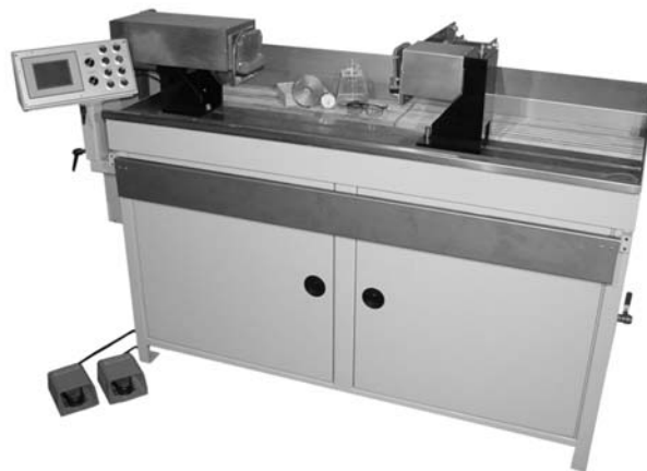
Figure B - Typical 2-vector multidirectional wet horizontal
