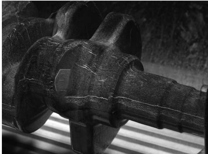
FIG. A1.4 Crankshaft with Various Longitudinal Indications
