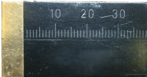
FIG. X2.3 One type of device containing a permanent magnet held next to two precision formed steel blocks with a brass cover. The seam between the steel blocks acts as a discontinuity; particles form an indication on the seam that is strongest close to the magnet and weakens with distance away from the magnet.
