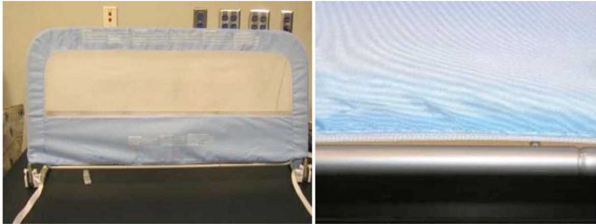
Bedrail fabric with bottom zipper misassembled, fabric cover can be zipped up without engaging the bottom horizontal bar.
