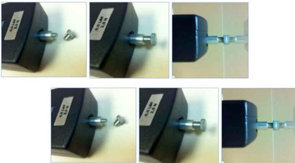
FIG. 3 Attaching the Force Gauge to Spray Disc
