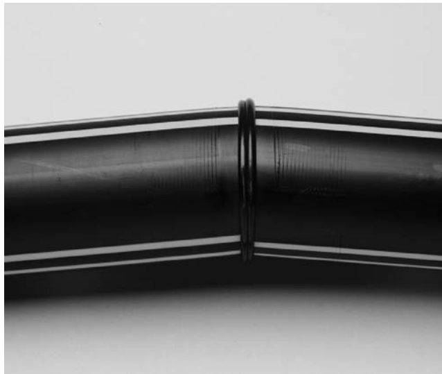
FIG. X2.10 Unacceptable Visual Appearance Butt Fusion
