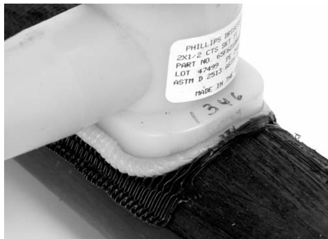
FIG. X2.14 Unacceptable Visual Appearance Saddle Fusion Joint
