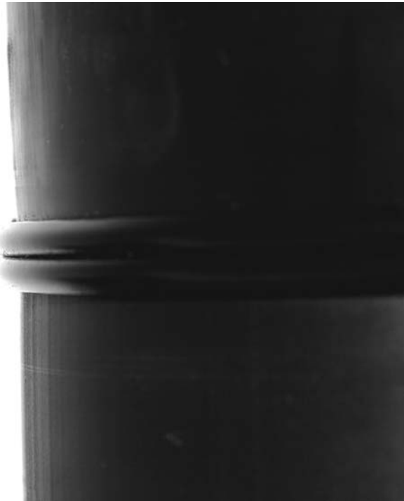
FIG. X2.6 Acceptable Visual Appearance Butt Fusion
