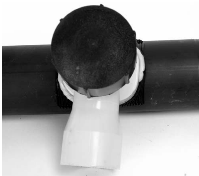
FIG. X2.13 Unacceptable Visual Appearance Saddle Fusion Joint
