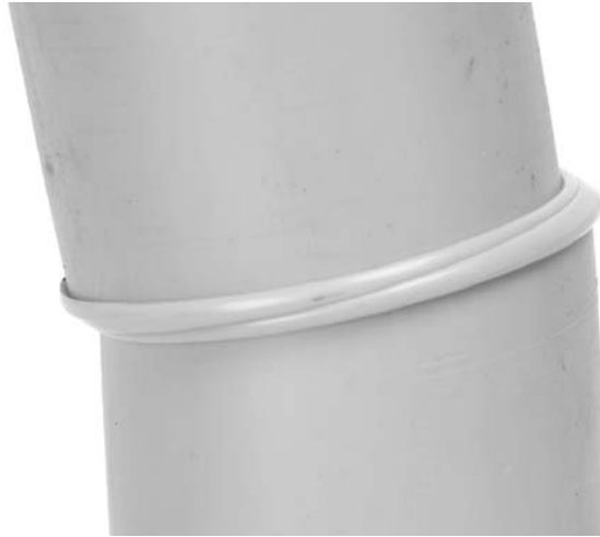
FIG. X2.9 Unacceptable Visual Appearance Butt Fusion
