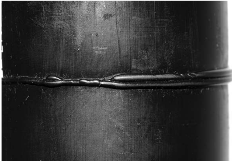
FIG. X2.7 Unacceptable Visual Appearance Butt Fusion
