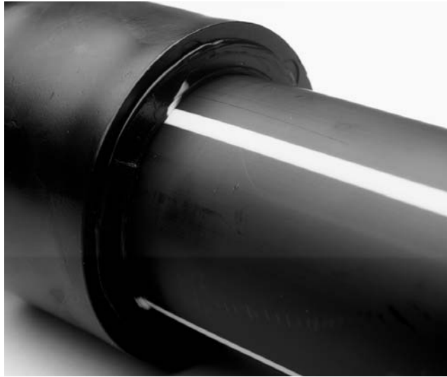
FIG. X2.1 Acceptable Visual Appearance Socket Fusion
