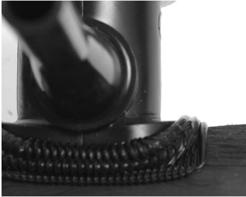
FIG. X2.14 Unacceptable Visual Appearance Saddle Fusion Joint
