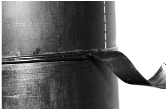
FIG. X2.11 Unacceptable Visual Appearance Butt Fusion
