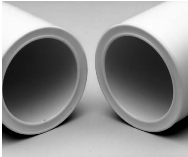
FIG. X2.8 Unacceptable Visual Appearance Butt Fusion
