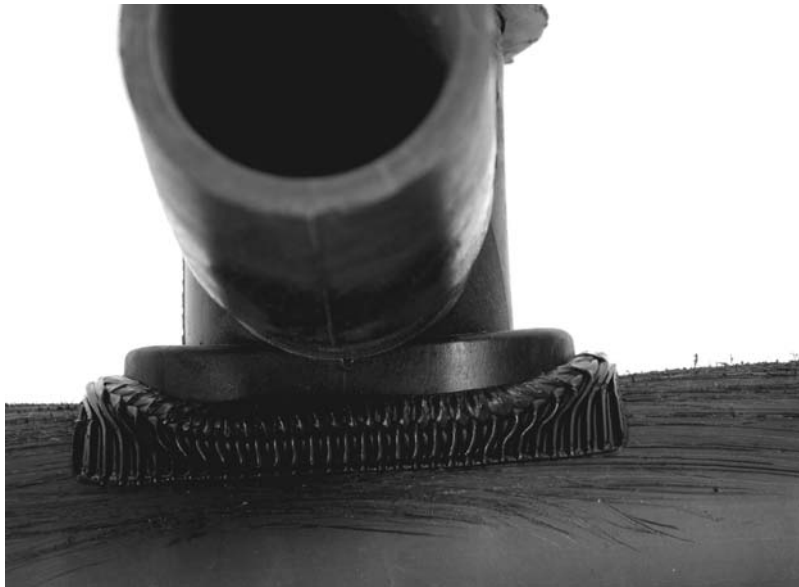
FIG. X2.12 Acceptable Visual Appearance Saddle Fusion Joint
