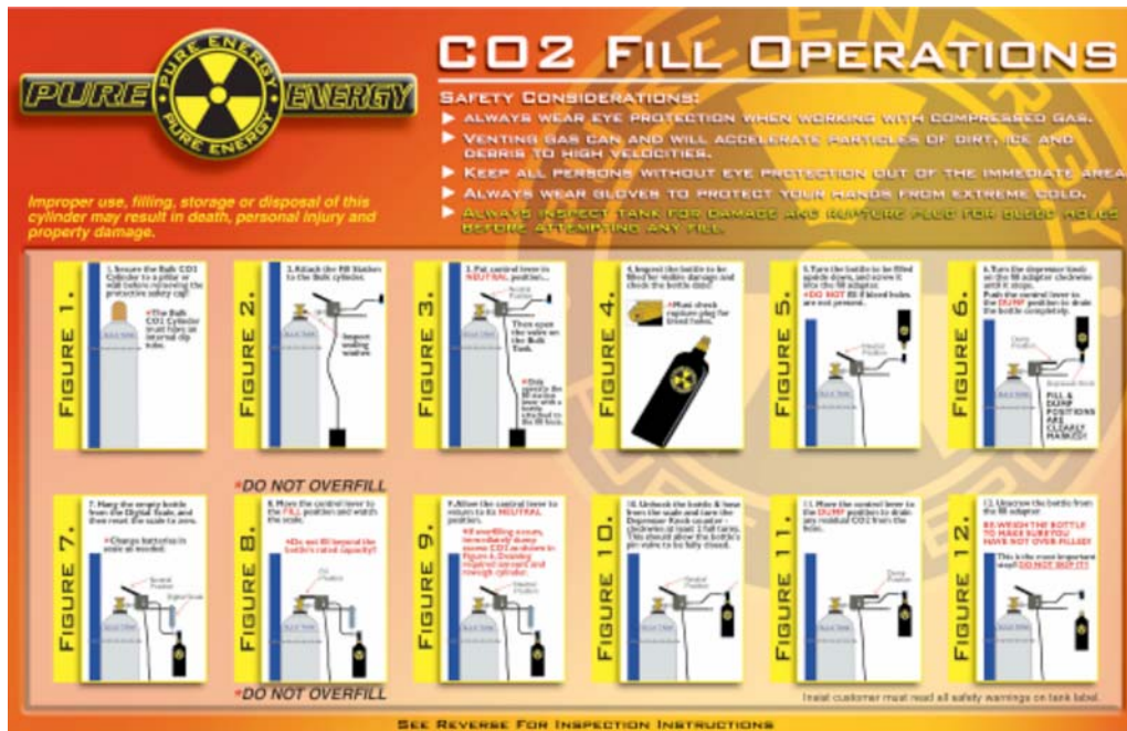
FIG. 3 Example of Fill Station Instruction Sheet A
