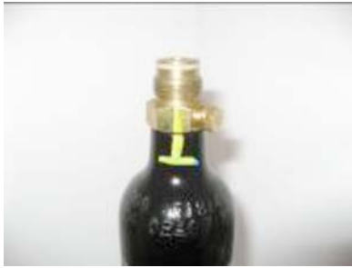
FIG. 6 Valve/Cylinder Rotation Indicator Marking
