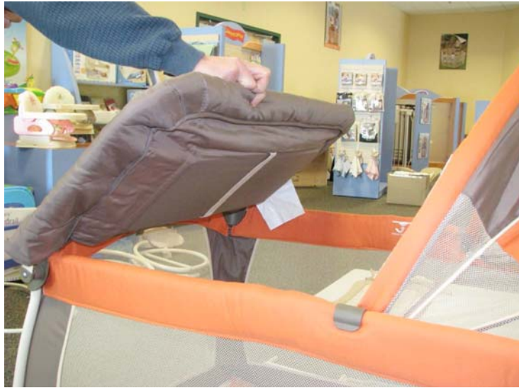
FIG. A1.5 Accessory That Attaches to the Play Yard on one Side and has Attachment Points that Rest on the Play Yard on the Other Side
