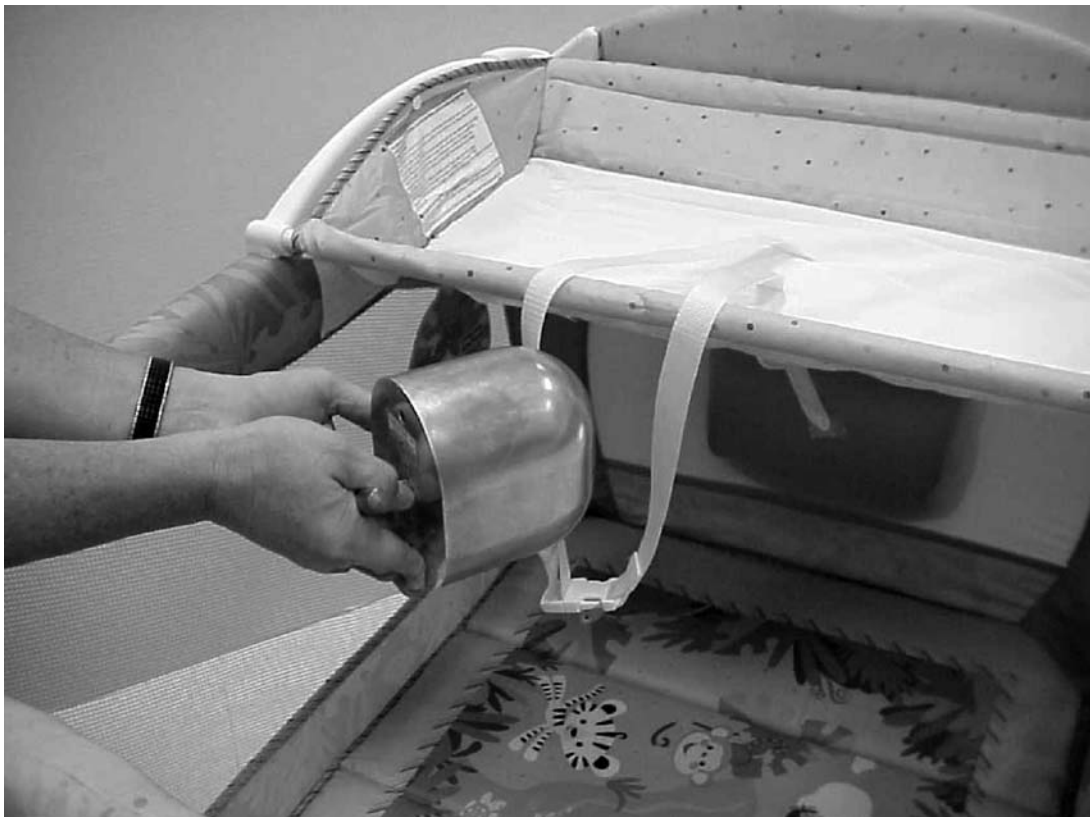
FIG. A1.10 Entrapment in Restraint Straps
