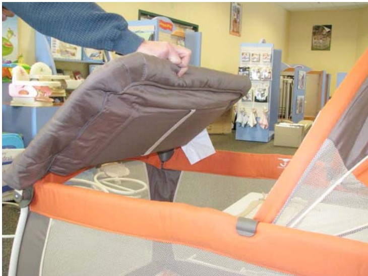
FIG. A1.6 Accessory That Attaches to the Play Yard on one Side and Rests on the Play Yard on the Other Side
