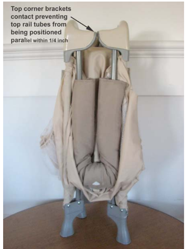
FIG. A1.33 Example of Folded Product whose Top Rails cannot be Made Parallel
