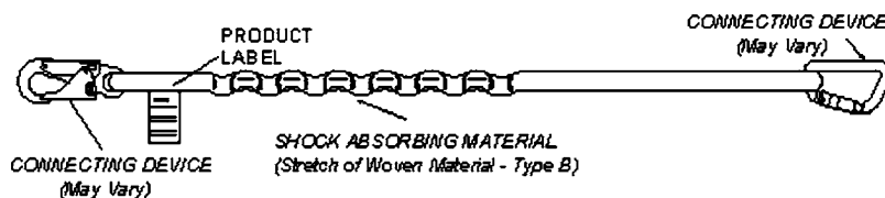
FIG. 28 Type "B" Shock Absorbing Lanyard
