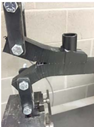
FIG. A2.4 Ductile Failure between Wires-Passing Result
