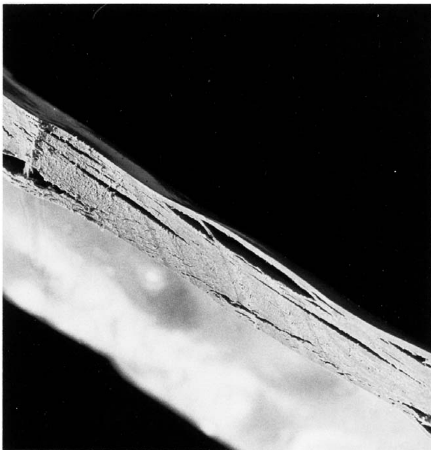
FIG. X1.2 Severe Wall Separation
