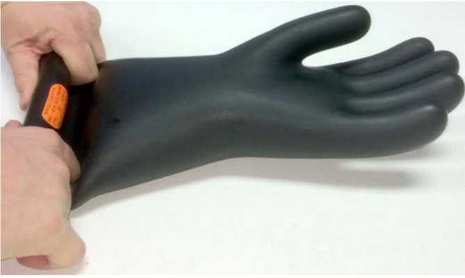
FIG. 44 Rolling – Trapping the Air
