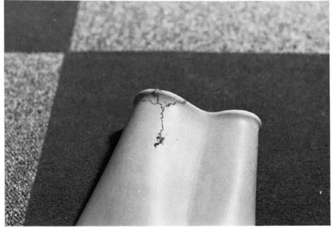
FIG. 29 Tracking—Insufficient Immersion Depth
