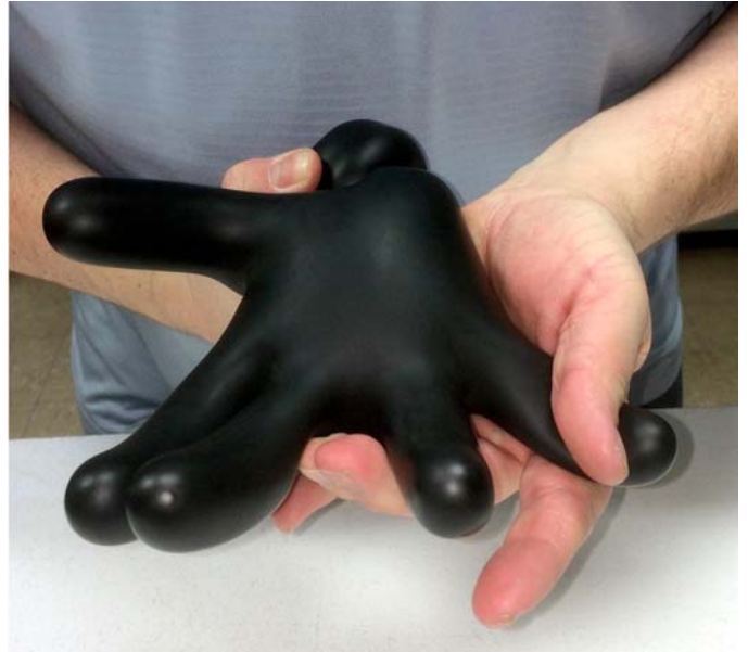
FIG. 35 Inspection – Between Fingers/Twirled Glove
