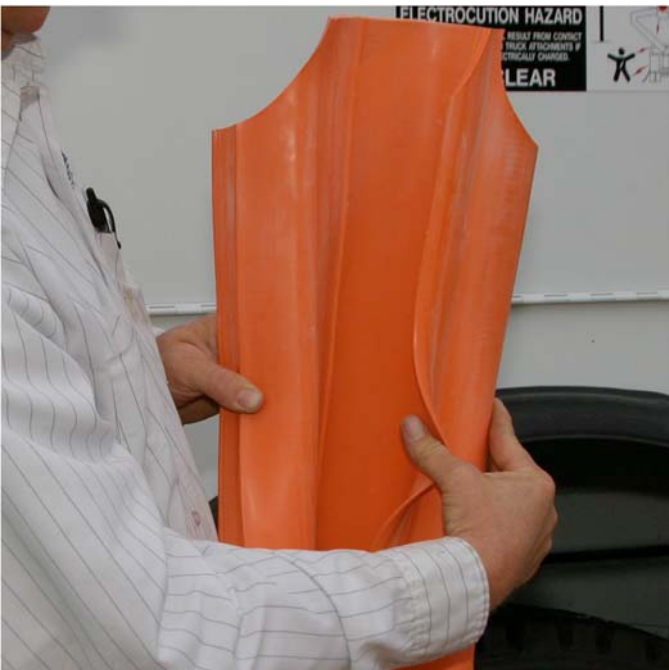
FIG. 37 Inspection – Inside Line Hose
