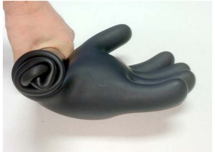
FIG. 46 Inspection – 14 in. Glove Length
