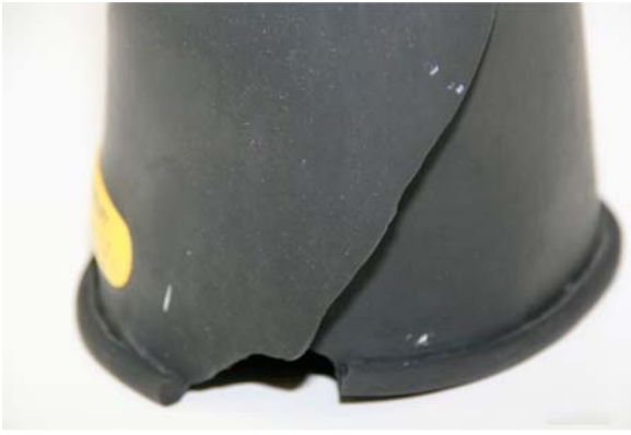
FIG. 26 Tear Rubber Glove
