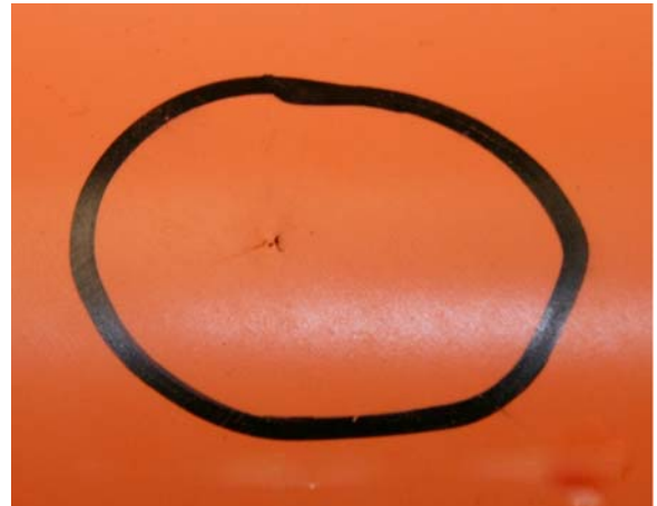
FIG. 5 Breakdown (Dielectric Failure Blanket: Front)
