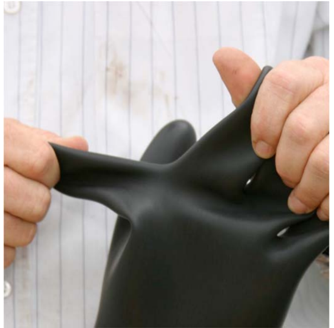
FIG. 34 Inspection – Between Fingers
