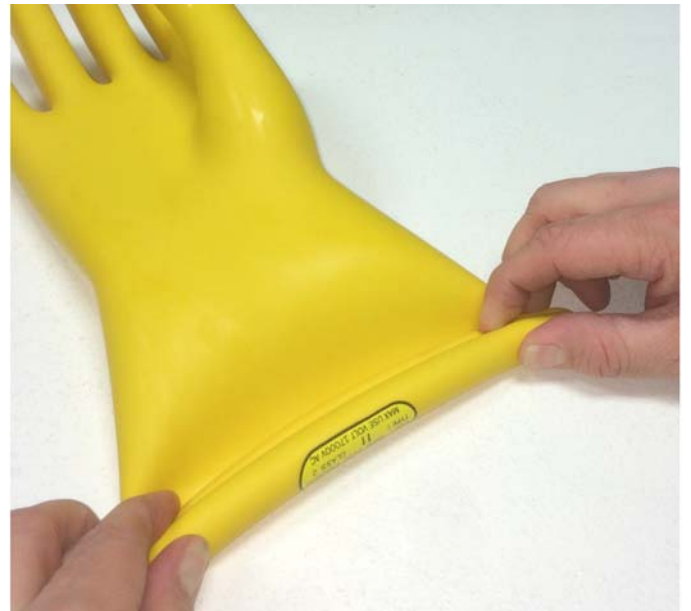
FIG. 43 Rolling – Sealing the Edges
