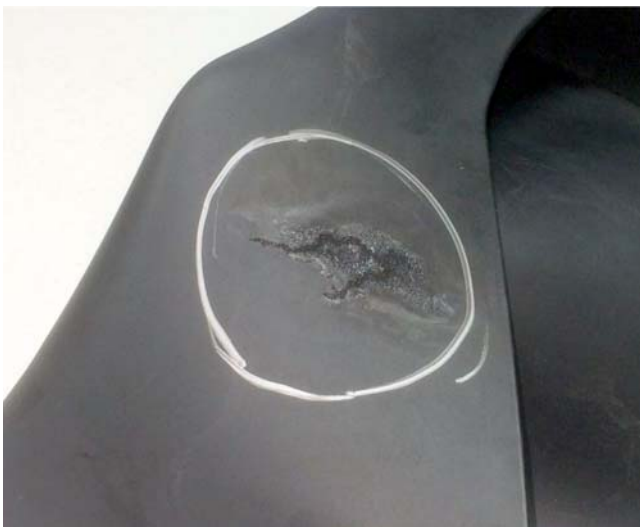
FIG. 28 Tracking—Burned Rubber Sleeve
