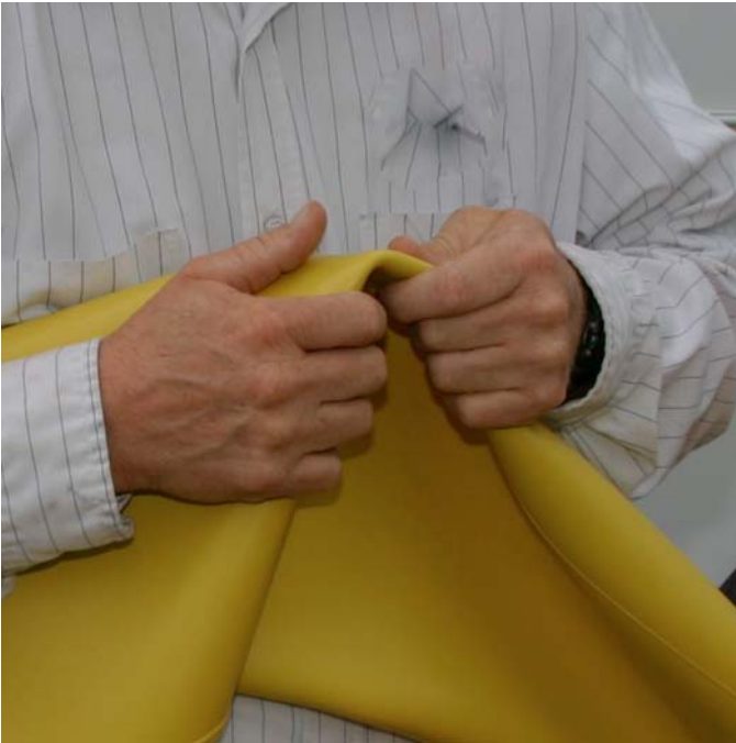
FIG. 31 Inspection – Sleeve Pinch Rolling
