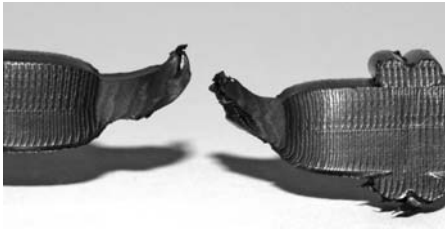
FIG. 2 Ductile Rupture Outside Fusion Interface
