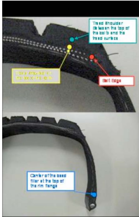
FIG. X1.1 Thermocouple Locations for Internal Tire Temperature Measurements
