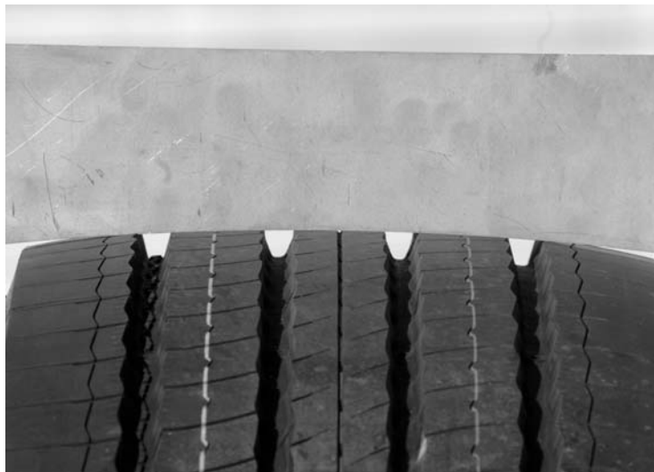
FIG. 4 Measuring a Tread Radius using a Reference Radius Template
