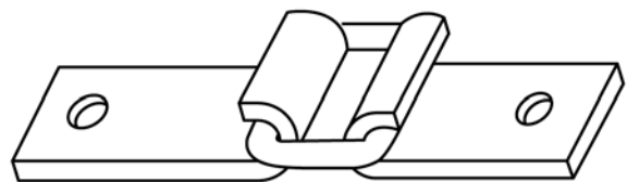
FIG. 21 Maximum Permanent Buckle Deformation Test
