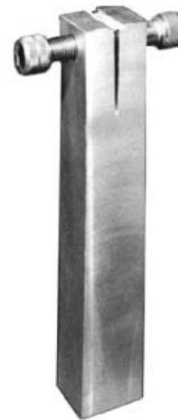
FIG. 4 Bolt Loaded Precracked Double Beam Specimen
