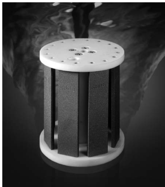
FIG. 2 Photo of Rotating Cage Containing Coupons
