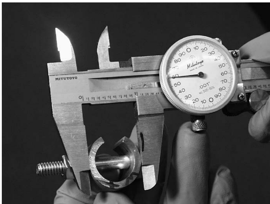
FIG. 4 Caliper Measurement of C-ring's Deflection
