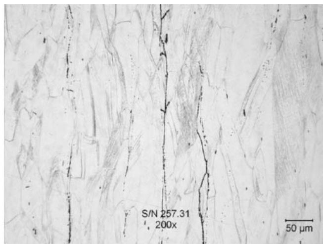
(h) 200X Original Magnification, Rejectable
