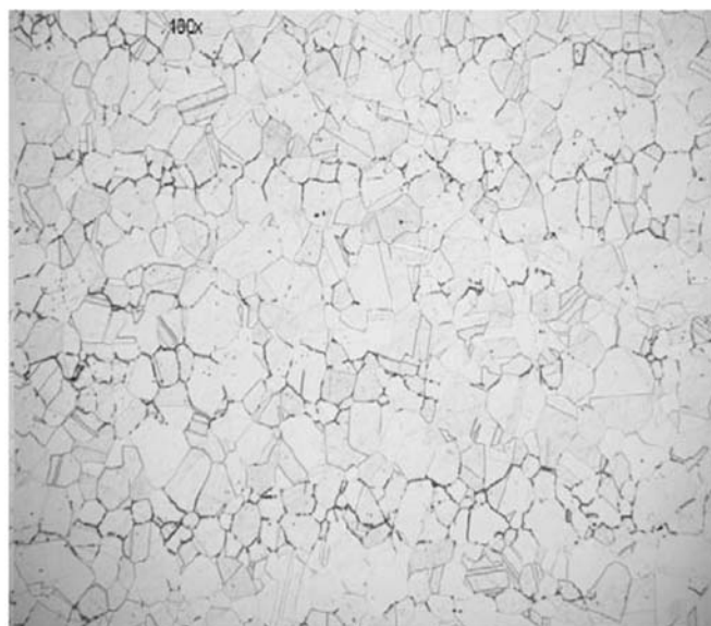
(b) 100X Original Magnification, Rejectable
