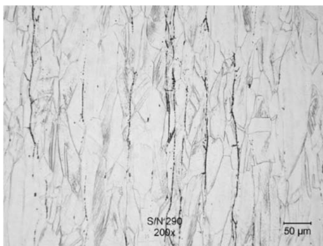
(i) 200X Original Magnification, Rejectable
