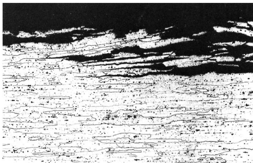
FIG. 2 Four Degrees of Severity of Exfoliation Corrosion
