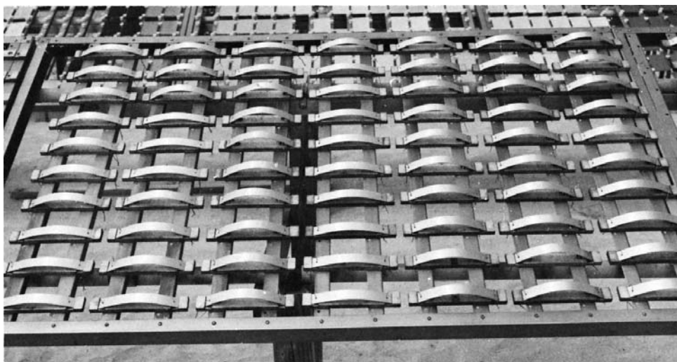
FIG. 4 Bent-Beam Specimens on Atmospheric Exposure Rack
