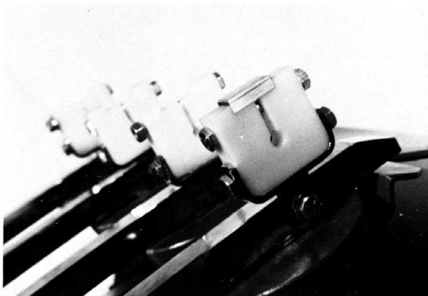
FIG. 5 Wear Block/Wear Specimen Holder
