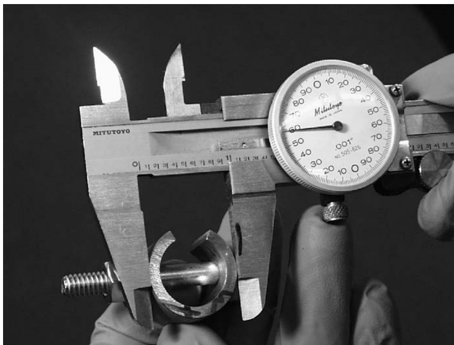
FIG. 4 Caliper Measurement of C-ring's Deflection
