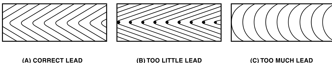
Figure 11—Effect of Lead Position on Bead Solidification Lines
