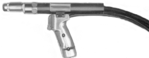
(B) WATER-COOLED PISTOL-GRIP GUN FOR PUSH WIRE FEED
