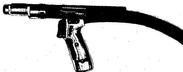
(B) PISTOL-GRIP GUN FOR PUSH WIRE FEED
