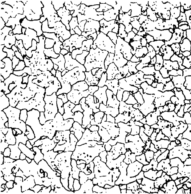
Photomicrograph of commercially pure iron, nominally called ferrite. No carbides are present, the acid etch reveals grain boundaries. The dark globules are nonmetallic inclusions.
