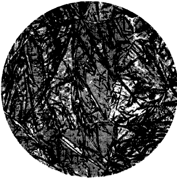
Quenched martensite (500X etched), showing acicular structure
