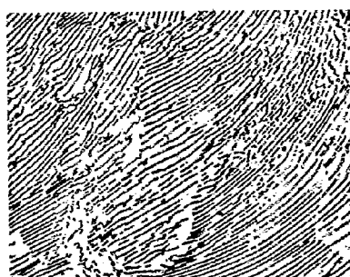
Fig. 7.2—Typical thin-layered structure of pearlite at 1500× (before reduction)
