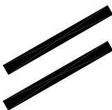
Figure 2 — Symbol for inclined joint
