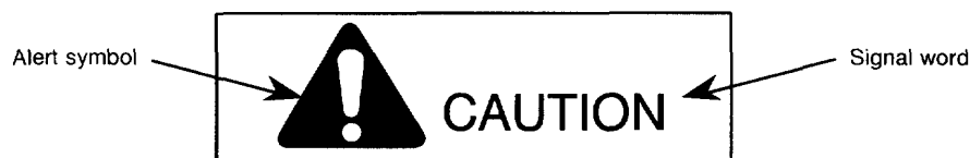
Fig. 3 Arrangement in signal panel (Example)
