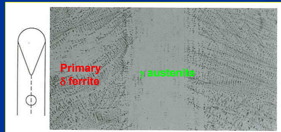
Section of F-Cr-Ni phase diagram showing change in solidification from ferrite to austenite due to dendrite tip undercooling
