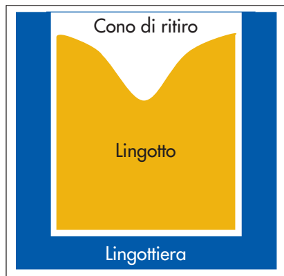
Figure 2 Schematic: Shrinkage cavity (primary pipe) on top of a cast ingot
