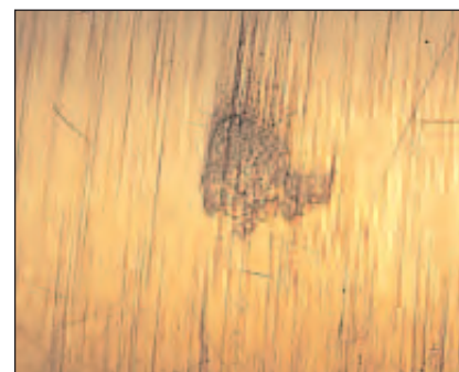
Fig. 20.3 14ct yellow gold made from contaminated gold
