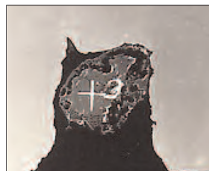
Fig. 13.4 Inclusion of slag with smooth edges, suggesting that the particle was probably liquid at the moment of casting
