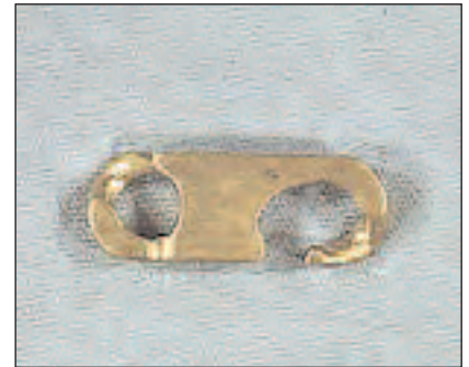
Fig. 14.1 A spring hook with surface porosity
