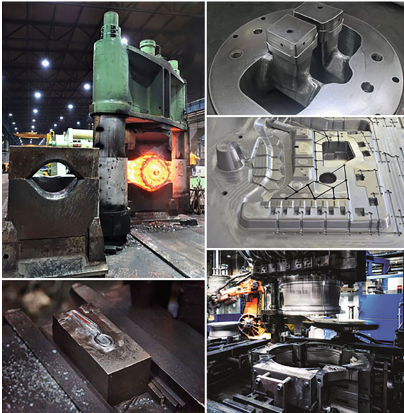
Fig. 5.2 Mosaic of selected applications of hot work tool steels, top left : forging saddles of a 2000-ton press (photo: Schlegel, J., BGH Edelstahl Lippendorf GmbH), bottom left : hammer die for a scissor piece (photo: Beck, K.-P., Bergheim), top right : extrusion die (photo: VT vetimec, dies & special components), middle right : die casting tool (photo: VT vetimec, dies & special components), bottom right : low-pressure casting tool for aluminum wheels (photo: Borbet GmbH)
