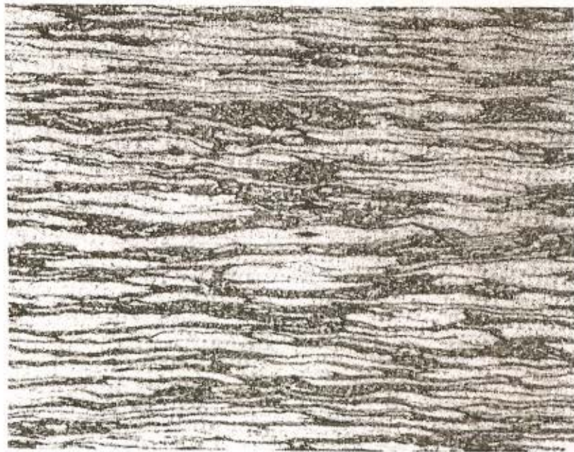
Figure 2-10 The microstructure of a typical duplex stainless steel. (Courtesy of Dr. E. V. Bravenec, Anderson & Assoc.)
