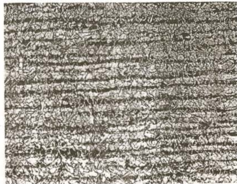
Figure 3-13 A banded ferrite-pearlite microstructure in carbon steel plate. (Courtesy of Dr. E. V. Bravenec, Anderson & Assoc.)
