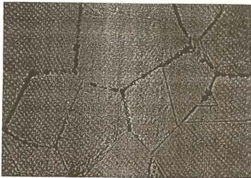
Figure 3-2 Sensitized Type 304 stainless steel. (Courtesy of Dr. E. V. Bravenec, Anderson & Assoc.)
