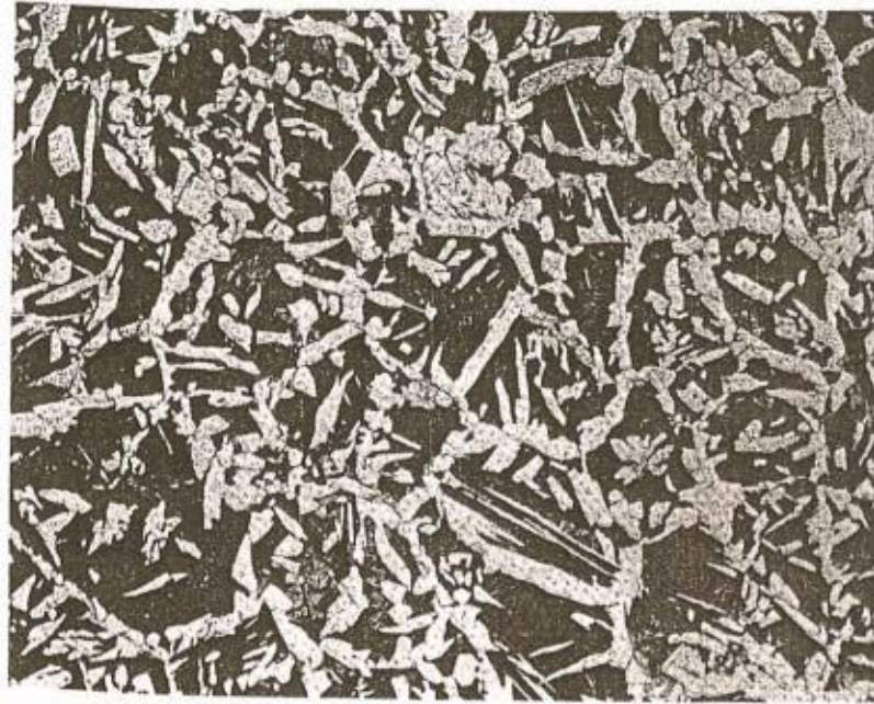
Figure 2-3 A typical microstructure in carbon steel that has been furnace annealed. (Courtesy of Dr. E. V. Bravenec, Anderson & Assoc.)
